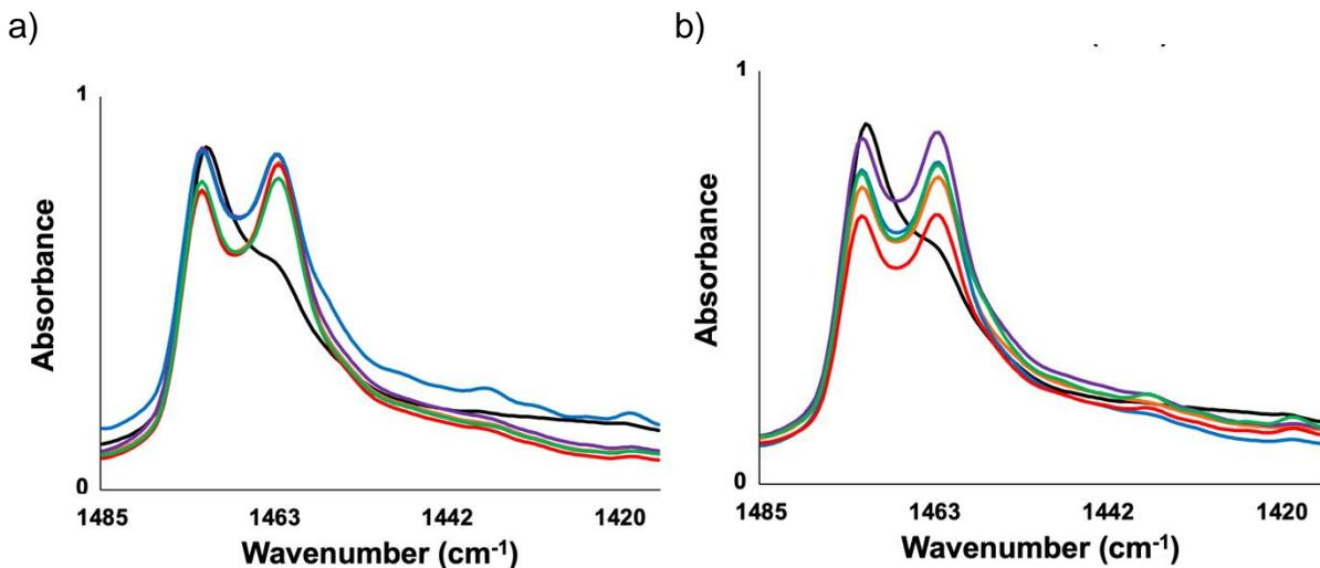
**Fig. 7.** FTIR spectrum of the surface of PE, showing the asymmetric rocking vibration of terminal methyl group in samples degraded by *P. ostreatus* grown in control medium (a) and in  $\text{H}_2\text{O}_2$  medium (b) in liquid fermentation. Control (black line), week 1 (orange line), week 2 (purple line), week 3 (blue line), week 4 (red line), and week 5 (green line).
