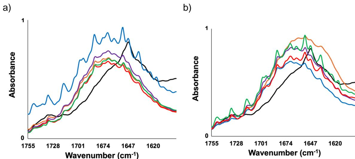
**Fig. 8.** FTIR spectrum of the surface of PE, showing the carbonyl group ( $1600\text{--}1750\text{ cm}^{-1}$ ) in samples degraded by *P. ostreatus* grown in control medium (a) and in  $\text{H}_2\text{O}_2$  medium (b) in liquid fermentation. Control (black line), week 1 (orange line), week 2 (purple line), week 3 (blue line), week 4 (red line), and week 5 (green line).
