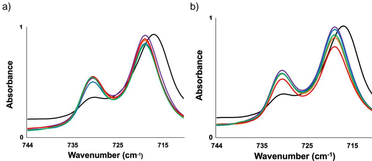
**Fig. 6.** FTIR spectrum of the surface of PE, showing the rocking vibrations of the methylene group in samples degraded by *P. ostreatus* grown in control medium (a) and in  $\text{H}_2\text{O}_2$  medium (b) in liquid fermentation. Control (black line), week 1 (orange line), week 2 (purple line), week 3 (blue line), week 4 (red line), and week 5 (green line).
