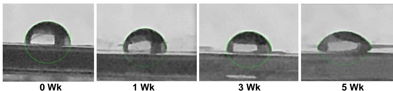
**Fig. 5.** Digital images showing a drop of water on the PE sample surface. The angle formed between the water drop and sample was measured (i.e. contact angle) to determine the hydrophobicity of the surface of PE after *P. ostreatus* growth in control medium (a) and in H<sub>2</sub>O<sub>2</sub> (b) at week 0, 1, 3 and 5 of fermentation.
