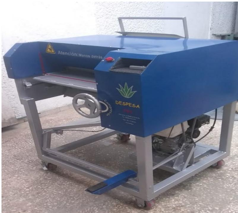
**Fig. 1.** Decortication machine adapted to *A. salmiana* leaves. This machine was provided with a set of adjustable pressing rollers before the scraping drum. Each agave leaf was squeezed by the operator through the pressing rollers to reduce leaf thickness down to 2 cm yielding abundant agave juice. Later, each squeezed leaf was scrapped by a revolving drum provided with transversal blades to separate the fiber from the pulp.
